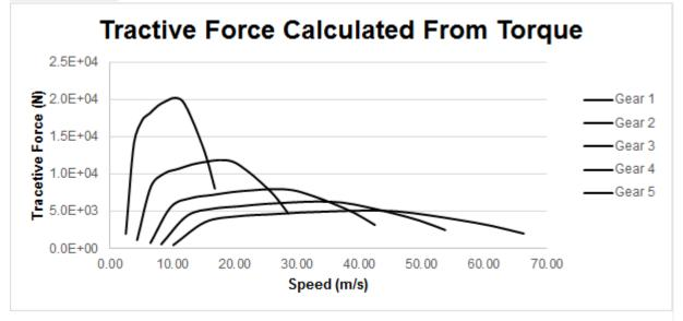
As you can see both power and torque methods produce exactly the same traction curves, so it really doesn't matter which one you use. You can simply pick the most convenient method based on the information available at the time.
