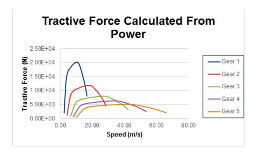
This gives a more accurate acceleration profile of the car both in each gear and throughout it's operating speed range.
